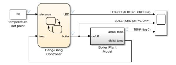
The example consists of a Stateflow chart and a Simulink® subsystem. The Bang-Bang Controller chart compares the current boiler temperature to a reference set point and determines whether to turn on the boiler. The Boiler Plant Model subsystem models the dynamics inside the boiler, increasing or decreasing its temperature according to the status of the controller. The boiler temperature then goes back into the controller chart for the next step in the simulation.
