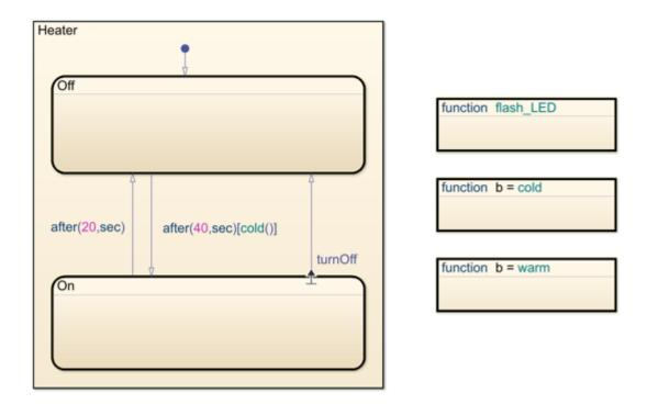
The labels on the transitions between the 0n and 0ff substates define the behavior of the bang-bang controller.
